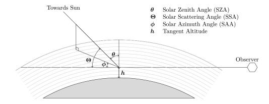
**Figure 1.** The limb viewing geometry and definitions of solar zenith angle, solar azimuth angle, solar scattering angle, and tangent altitude. The tangent altitude and solar zenith angles are defined relative to the un-refracted tangent point. Figure adapted from Zawada et al. (2015).
