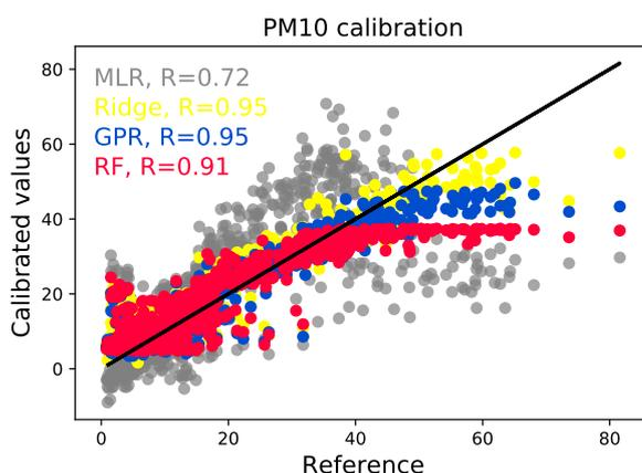
**Figure 6.** Calibrated PM10 values (in  $\mu\text{g m}^{-3}$ ) versus the reference measurements for 900 hours of test data at location CarPark for the  $I_{24}$  predictor set-up. The ideal 1:1 perfect prediction line is drawn in black. Inset values  $R$  are the Pearson correlation coefficients.
