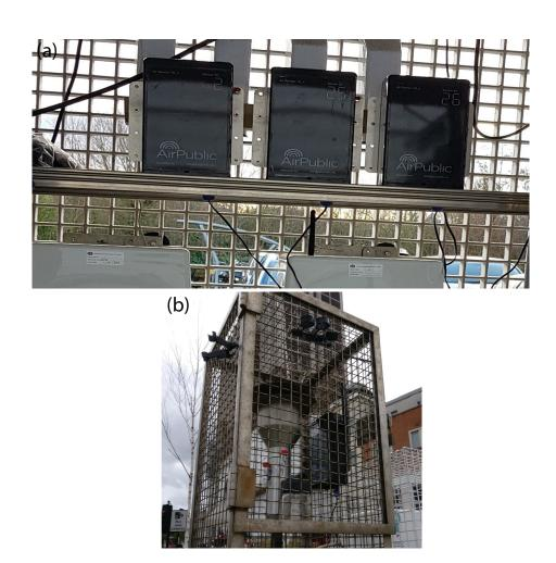
**Figure 2.** Examples of the co-location set-up of the AirPublic low-cost sensor nodes with reference measurement stations at sites (a) CarPark and (b) CR9, respectively.
