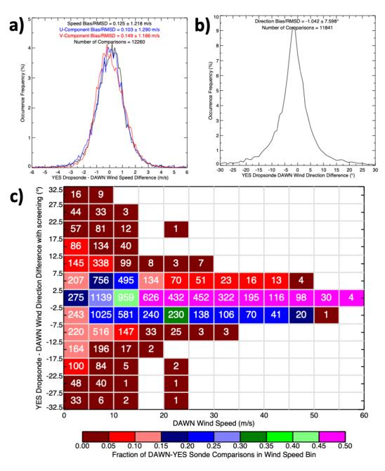
Figure 15: A comparison of DAWN and dropsonde vector wind speed (black), and u- and v-component speed (blue and
