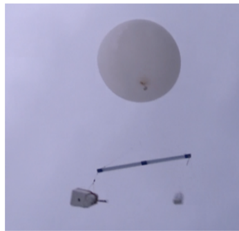
Figure 1. Photographs of the CPS sonde operation at the (a) RV Mirai in October 2019 and (b) Ny-Ålesund in March 2020. The CPS housing within a black inlet duct on top is connected to the Meisei RS-11G radiosonde. During the 2019 and 2020 campaigns, the Vaisala RS41-SGP was attached to the opposite side of the rod.
