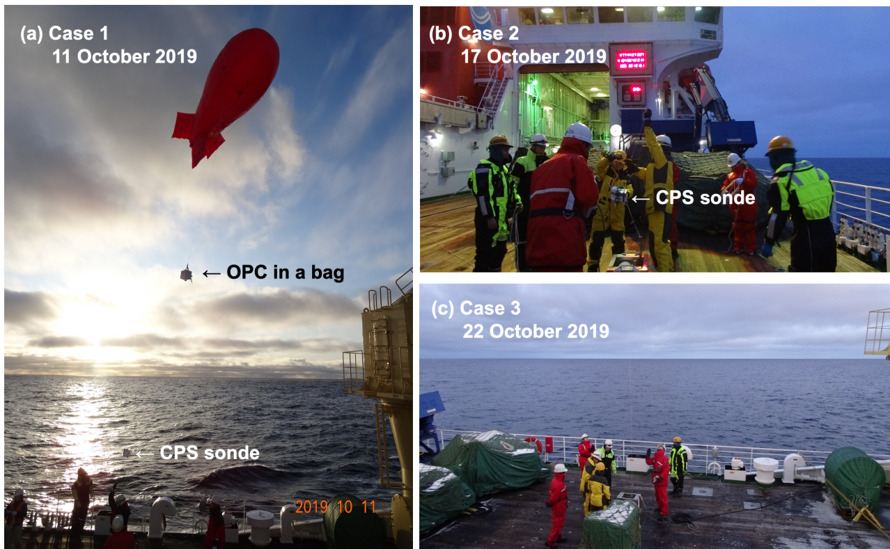
Figure 4. Photographs of tethered balloon measurements for the cases of (a) October 11, 2019 (MR19-CPST1), (b) October 17, 2019 (MR19-CPST2), and (c) October 22, 2019 (MR19-CPST3) on RV Mirai in the Arctic Ocean.
