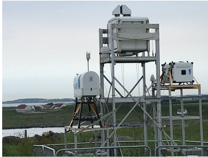
Figure 4. The main instrumental site of the COTUR campaign with one of the scanning lidars, Leosphere WindCube 100S (LidarN) in the center, the Leosphere WindCube v1 wind profiler to the right and the Radiometer Physics HATPRO RG4 passive microwave temperature and humidity profiler to the left. The picture is taken towards north-northwest.
