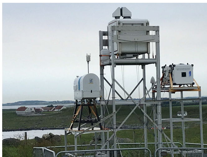
Figure 4. The main instrumental site of the COTUR campaign with one of the scanning lidars, Leosphere WindCube 100S (LidarN) in the center, the Leosphere WindCube v1 wind profiler to the right and the Radiometer Physics HATPRO RG4 passive microwave temperature and humidity profiler to the left. The picture is taken towards north-northwest.
