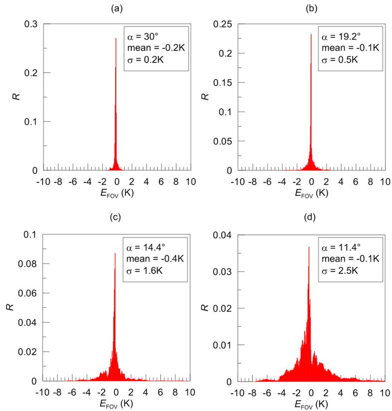
**Fig. D: Statistical distributions (in terms of relative frequency of occurrence  $R$ ) of brightness temperature difference  $E_{FOV}$  “ $T_B$  neglecting FOV minus  $T_B$  accounting for FOV” at 31.4 GHz simulated for four elevation angles. Input data: the Monte Carlo model of scattered clouds.**
