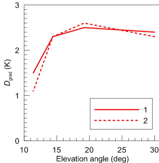
**Fig. C: The LWP gradient signal  $D_{\text{grad}}$  as a function of the elevation angle at 31.4 GHz. Input data: the Monte Carlo model of scattered clouds. Solid line (1) corresponds to the results obtained with account for FOV; dashed line corresponds to the results obtained when FOV is neglected.**
