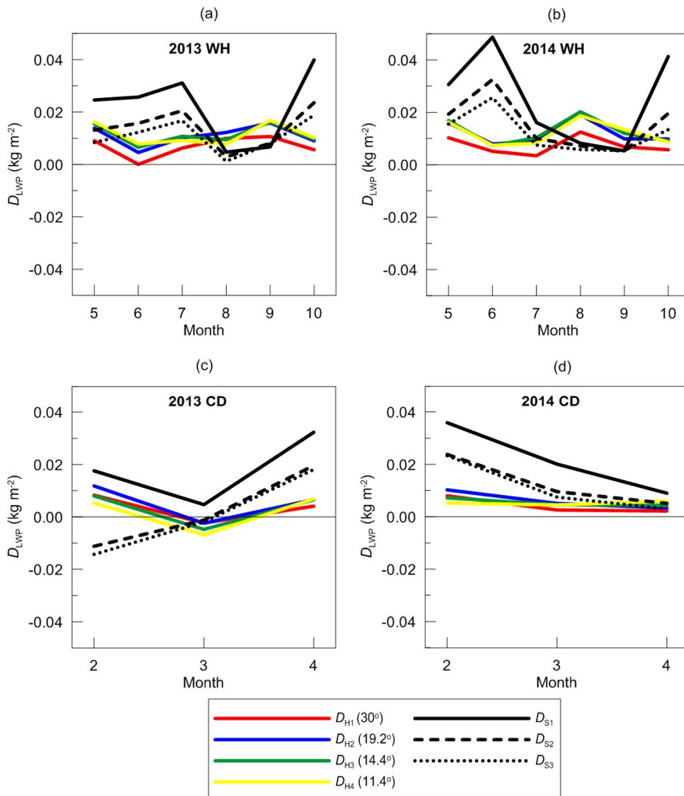
**Figure 12:** Monthly mean land-sea LWP difference  $D_{LWP}$  as a function of time for various time periods obtained from the satellite and the ground-based observations.  $D_{Hj}$  ( $j=1,\dots,4$ ) denote  $D_{LWP}$  obtained by the HATPRO instrument at four elevation angles (colour lines, see the legend).  $D_{Sj}$  ( $j=1,2,3$ ) denote  $D_{LWP}$  obtained by the SEVIRI instrument and calculated by three different formulae, see the text.
