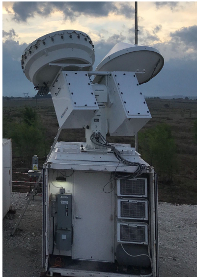
Figure 2. The Ka/X SACR deployed at the mobile facility outside of Villa Yacanto, Argentina. The radar is a dual frequency radar with two antennas mounted on a single pedestal.
