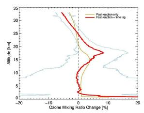
Figure 11: Median difference between corrected and originally reported ozone mixing ratio for 577 ozonesondes launched at Costa Rica. Thin orange line: removal of the slow reaction contribution only. Thick red line: complete correction algorithm including the time lag correction. The thin blue lines: One standard deviation around the complete correction algorithm.
