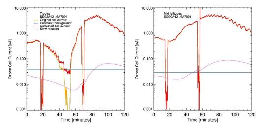
Figure 4: Cell current components of the tropical and mid-latitude simulations shown in Figure 3. Red lines: Fast cell current contribution. Puprle lines: Slow reaction contribution. Orange lines: Originally measured cell current minus constant background. Light blue lines: Constant background.
