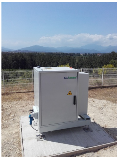
Figure 1. Mini Micro Pulse LiDAR (MiniMPL) unit from the Météo-France network.
