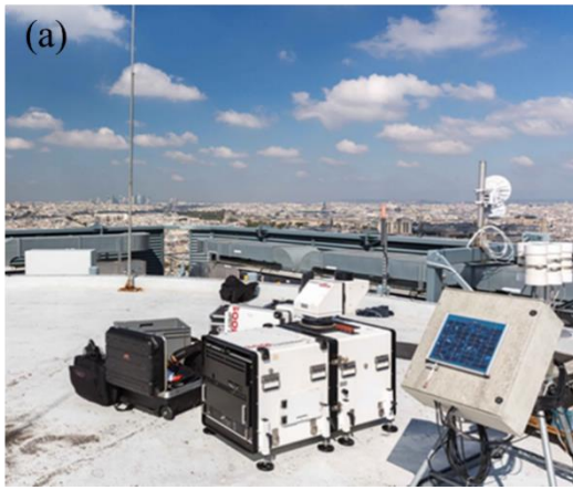
Figure 1: (a) The Doppler lidar installed on the tower roof during the VEGILOT campaign and (b) the measurement site in Paris with the circle of 10 km diameter demonstrating the maximum range of the PPI surface scan (Google earth satellite image).
