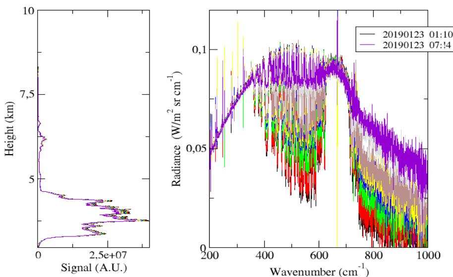
Page 12, Lines 243 – 244: The high liquid water optical depths likely fully attenuate the lidar signal which is why it is not reproducible using the Klett inversion.
