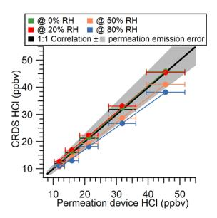
**Figure 2.** Comparison of CRDS HCl measurements and output from an HCl permeation device over a range of RHs. Error bars in the x direction represent propagated IC measurement error, while error bars in the y direction represent the standard deviation of online sampling plateau for each mixing ratio (low magnitudes mean these error bars do not extend beyond the points). A 1:1 correlation (solid black line) is shown with the uncertainty in the permeation device emission rate (shaded grey area).
