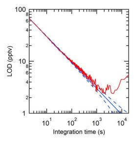
Figure 1. Allan-Werle deviation  $(3\sigma)$  in the optical cavity purged with zero-air (red line) shown with the ideal deviation (no drift, solid blue line) and associated error in the deviation (dashed blue line).
