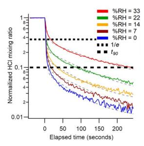
**Figure 4.** Background corrected and normalized signal decay curves observed for pulsed HCl (24 ppbv) performed at various RHs. Dashed grey lines represent a double exponential fit to the average of three cycles at each water mixing ratio. The short and long dashed black lines indicate 37 % (1/e) and 90 % ( $t_{90}$ ) decrease from the initial signal, respectively.
