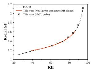
**Figure 2:** Hygroscopic growth of ammonium sulfate determined using a NaCl droplet as a probe of the RH. The points represent a measurement using discrete steps in RH, while the red line indicates a measurement where the RH was changed in 0.5% increments to achieve a pseudo-continuous change in RH. Both datasets agree with the E-AIM prediction of radial growth factor within 1%.
