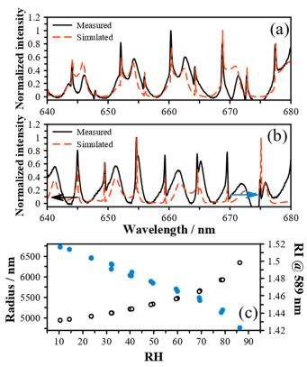
595 Figure 5: Measured spectra for a droplet of citric acid at: (A) high RH (~85%) with a radius of 6328 nm and a RI of 1.4225; (B) low RH (~10%) with a radius of 4954 nm and a RI of 1.5175. Both spectra are shown with the Mie theory simulation using these values as inputs. (C) The size and RI of a citric acid droplet as a function of RH determined using a LiCl probe.
