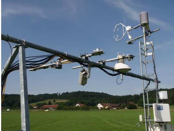
Figure 4: Photograph of the eddy-covariance system at DE-Fen grassland site. The hill in the background has a height of about 100 m compared to the grassland in the foreground (photograph by Matthias Mauder).
