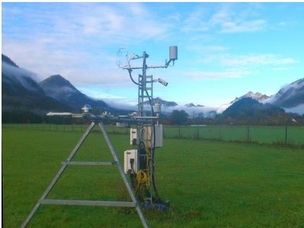
Figure 5: Photograph of the eddy-covariance system at DE-Gwg grassland site. The mountains in the background are up to 1000 m higher than the grassland in the foreground (photograph by Matthias Mauder).
