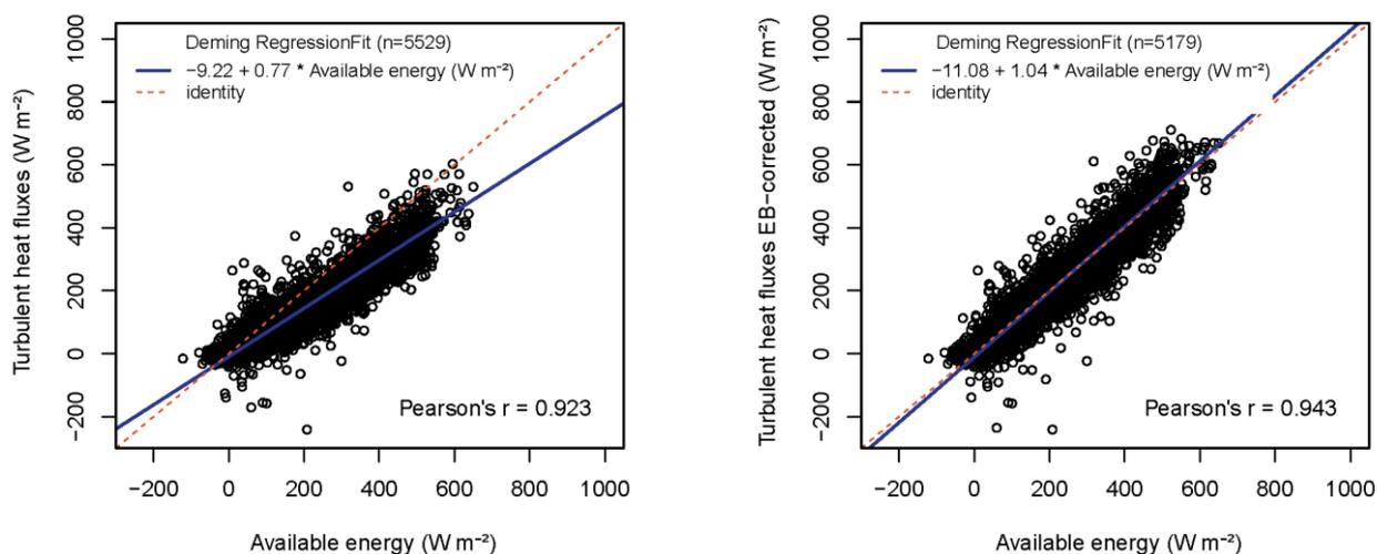
270 **Figure 8:** Results the orthogonal regression analysis of the sum of the turbulent heat fluxes ( $H + \lambda E$ ) vs. the available energy ( $R_n - G$ ) as measured (left panel) and after application of the EBC correction (right panel) for the DE-Fen dataset.
