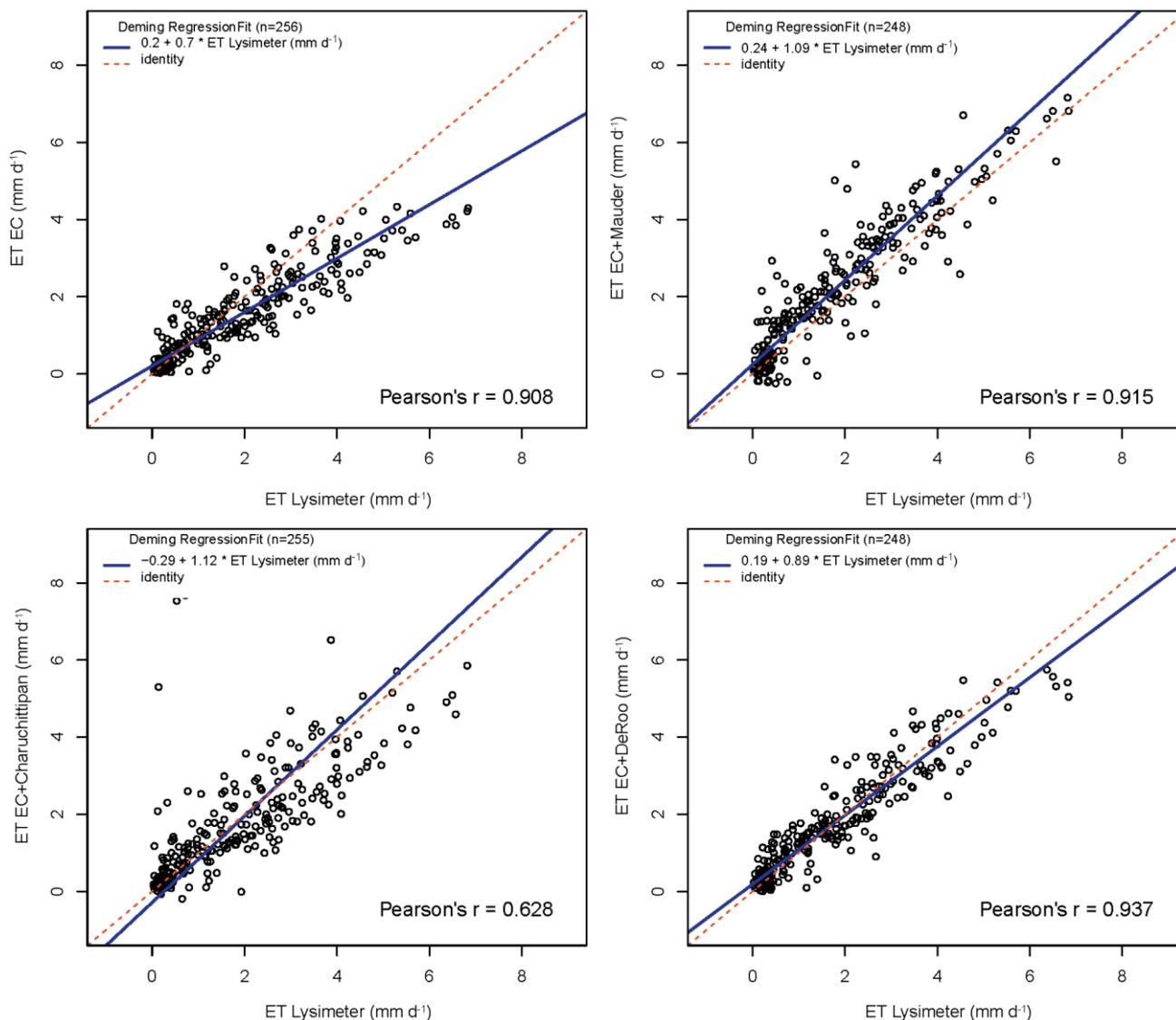
295 **Figure 10: Comparison of daily evapotranspiration (ET) estimates based on eddy-covariance measurements after different variants of energy balance closure correction with daily ET estimates based on lysimeter measurements for the DE-Fen dataset.**
