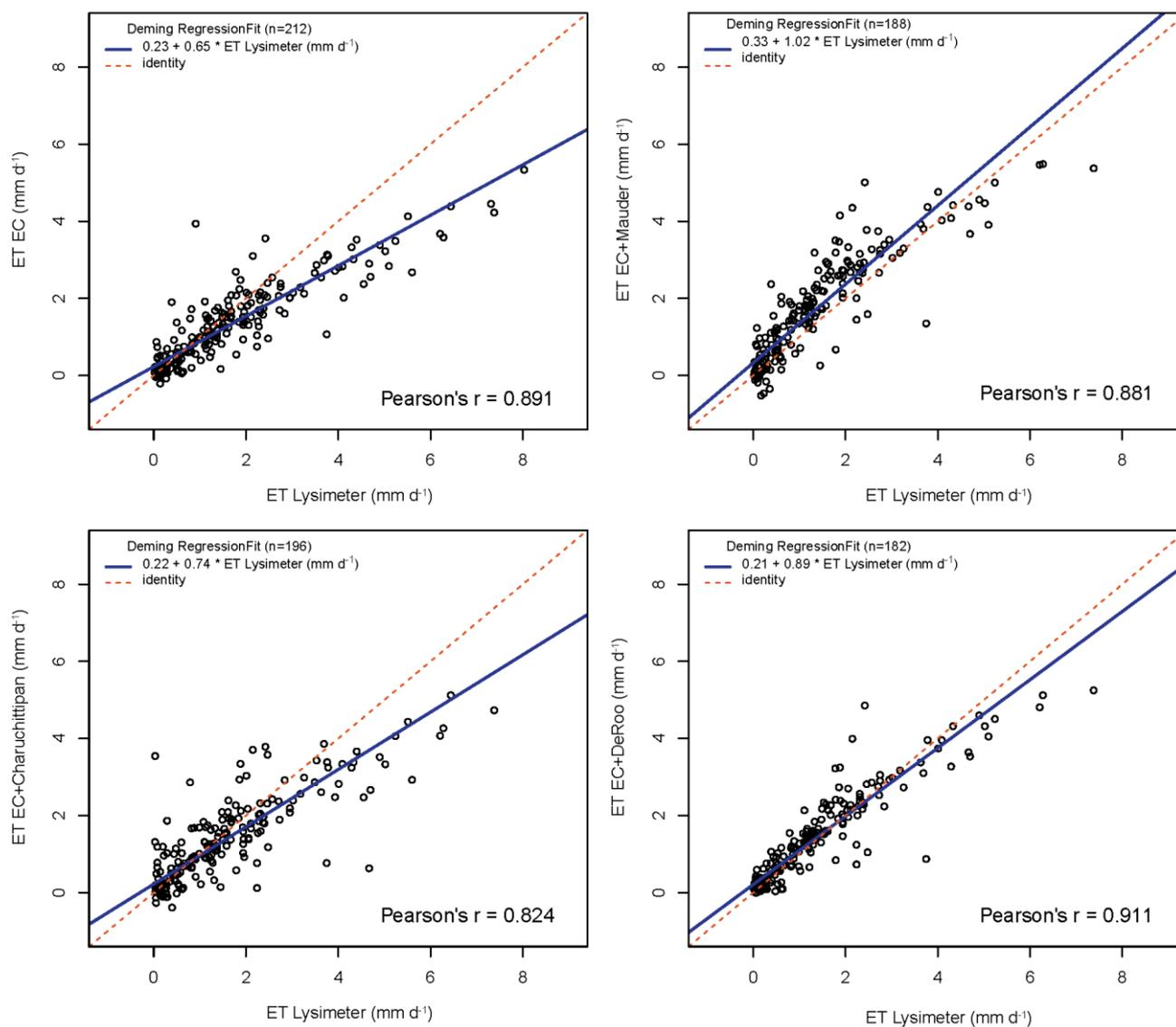
**Figure 11: Comparison of daily evapotranspiration (ET) estimates based on eddy-covariance measurements after different variants of energy balance closure correction with daily ET estimates based on lysimeter measurements for the DE-Gwg dataset.**
