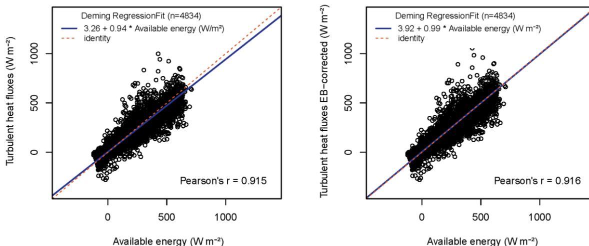
**Figure 6: Results of the orthogonal regression analysis of the sum of the turbulent heat fluxes ( $H + \lambda E$ ) vs. the available energy ( $R_n - G$ ) as measured (left panel) and after application of the EBC correction (right panel) for the DK-Sor dataset.**
