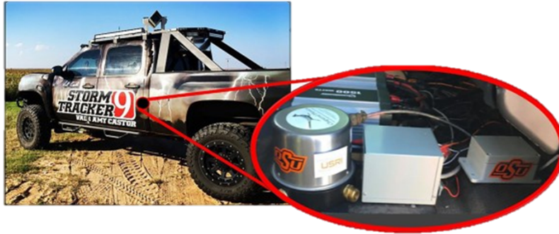
Figure 2. Image of GLINDA-housing storm chasing vehicle showing approximate location and configuration of install.
