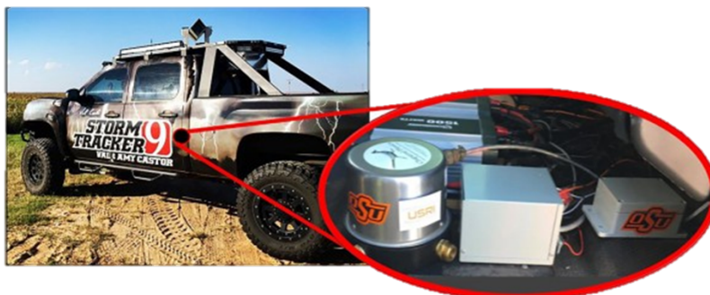
Figure 2. Image of GLINDA-housing storm chasing vehicle showing approximate location and configuration of install.
