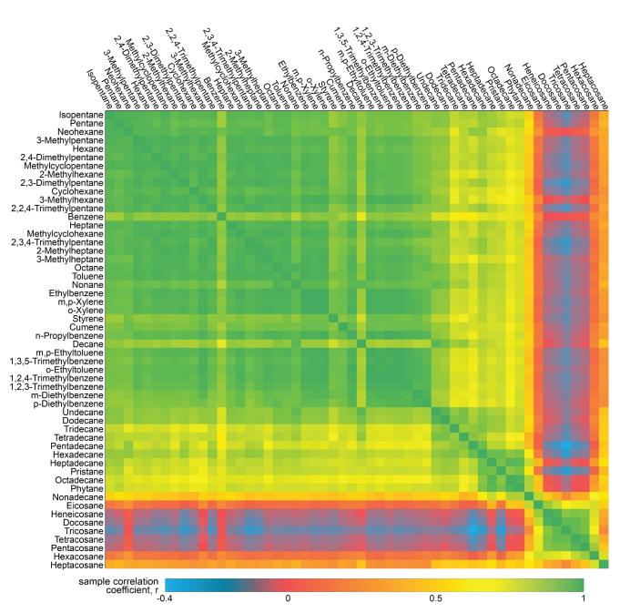
**Figure 9** Pearson's R correlation matrix for a suite of petroleum-derived compounds observed by cTAG in Livermore, California between April 11<sup>th</sup> and April 21<sup>st</sup>, 2018, ordered by volatility. Two distinct groupings emerge from  $C_5$  alkane-equivalent volatility to  $C_{11}$  and  $C_{20}$  to  $C_{26}$ , with a third less distinct but still prominent grouping from  $C_{11}$  to  $C_{19}$ .
