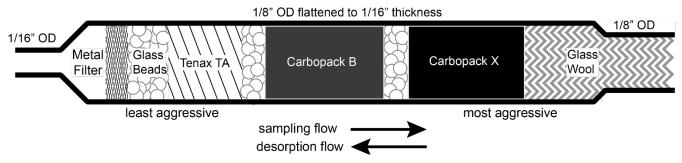
**Figure 2** Schematic of I/VOC collector. Semivolatile and lower volatility species, including particles, are captured on the metal filter. IVOCs are captured on the glass beads and Tenax TA, while the most volatile analytes including isoprene are retained by the more aggressive adsorbents. Flow is reversed for desorption so that the less volatile compounds never interact with the more aggressive adsorbents.
