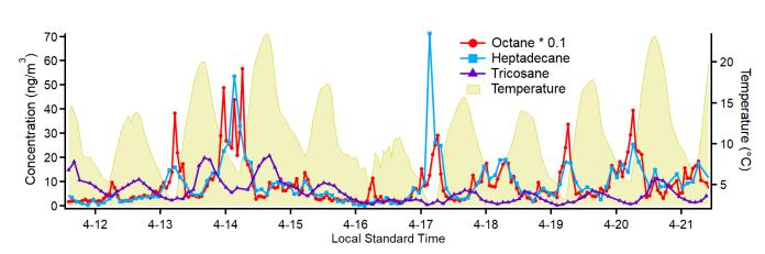
**Figure 10** Timelines for characteristic species from each of the three main groupings of compounds evident in the correlation matrix (Fig. 9). The two more volatile groups, represented by octane and heptadecane, tend to peak in the early morning, consistent with morning rush hour cold start emissions. The least volatile group, which includes tricosane, appears to have an evaporative source as it tracks closely, but slightly delayed, with ambient temperature.
