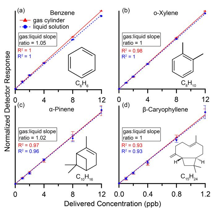
**Figure 4** Calibration curves with  $R^2$  values for (a) benzene, (b) o-xylene, (c)  $\alpha$ -pinene and (d)  $\beta$ -caryophyllene in a gas cylinder (red) and in a custom liquid mixture (blue), delivered by the dynamic dilution system (Fig. 3). Normalized detector response on the y-axis is the integrated area of the chromatographic peak divided by that of neohexane, our internal standard, on the same chromatogram. Maximum normalized
