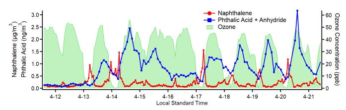
Figure 8 Concentration timelines for naphthalene, a primary emission from vehicle exhaust measured on cTAG's I/VOC channel, and the sum of phthalic anhydride and phthalic acid, secondary photooxidation products of naphthalene detected on cTAG's SVOC channel. Another secondary compound, ozone, measured at a nearby Bay Area Air Quality Management District monitoring site, provides an independent indication of photochemical activity.
