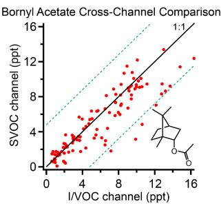
**Figure 6** Bornyl acetate measured on the I/VOC and SVOC channels of cTAG during FIREX-AQ. Dashed lines represent  $\pm 4.8$  ppt (3 times the I/VOC channel limit of detection for bornyl acetate). 96 % of data points fall within the region bounded by the dashed lines. R<sup>2</sup> is 0.79.
