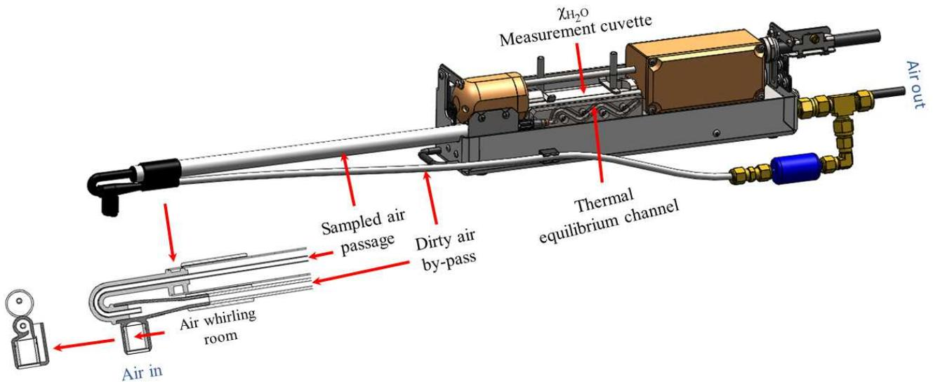
330 **Figure 3: Vortex intake system for air flow through its individual compartments: Air whirling room (2.200 mL), sampled air passage (1.889 mL), thermal equilibrium channel (0.587 mL), and  $\chi_{H_2O}$  measurement cuvette (5.887 mL). The internal space of all compartments adds up to a total volume of 10.563 mL.**
