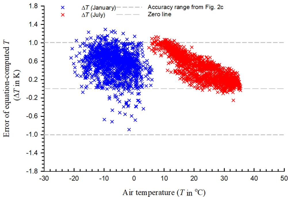
**Figure 4:** The error of equation-computed  $T$  in the coldest (January) and hottest (July) months of 2019 in Logan, UT, USA.  $\Delta T$  is equation-computed minus RTD-measured  $T$ , where RTD is a precision platinum resistance temperature detector inside a fan-aspirated radiation shield.  $\Delta T$ :  $0.549 \pm 0.281\text{ K}$  in January and  $0.436 \pm 0.290\text{ K}$  in July. See Fig. 2c for the accuracy range.
