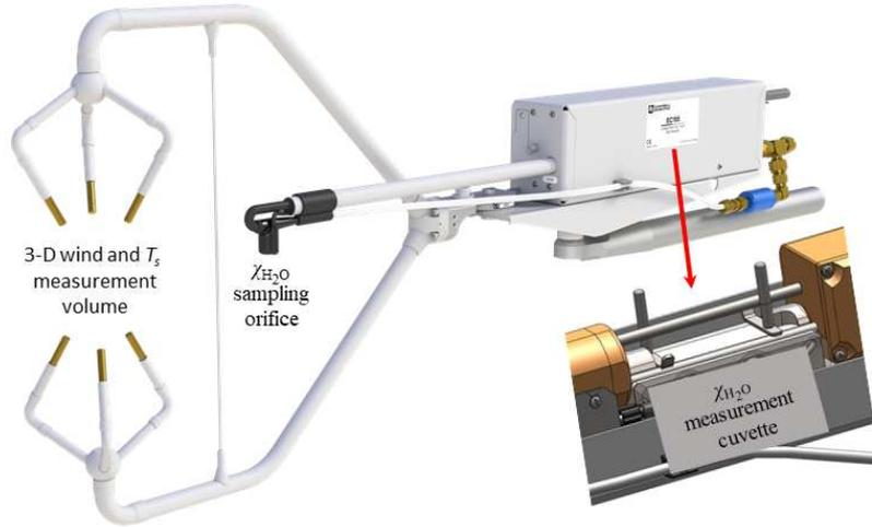
65 **Figure 1: Measurement volume for three-dimensional (3-D) wind and sonic temperature ( $T_s$ ), sampling orifice for  $\text{H}_2\text{O}$  molar mixing ratio ( $\chi_{\text{H}_2\text{O}}$ ), and measurement cuvette for  $\chi_{\text{H}_2\text{O}}$  in CPEC300 series (Campbell Scientific Inc., UT, USA).**
