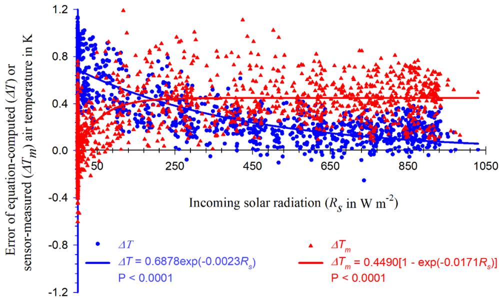
**Figure 6: Errors in equation-computed and sensor-measured air temperature ( $T$ ) with incoming solar radiation.  $\Delta T$  is equation-computed minus RTD-measured  $T$ , where the RTD is a precision platinum resistance temperature detector inside a fan-aspirated radiation shield.  $\Delta T_m$  is sensor-measured minus RTD-measured  $T$ , where the sensor is a HMP155A air temperature and humidity probe inside a wind-aspirated radiation shield.**
