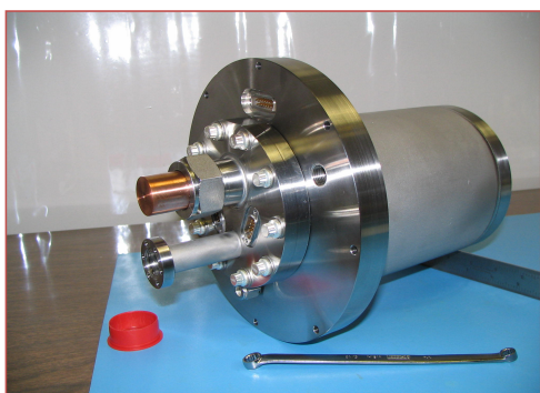
475 Figure 1: Top left is the cold finger that is held at 20° C. Top right is the CCD detector that mounts on the copper cold finger. Bottom left and right are the back and front of the assembled housing. The CCD detector is behind the window.
