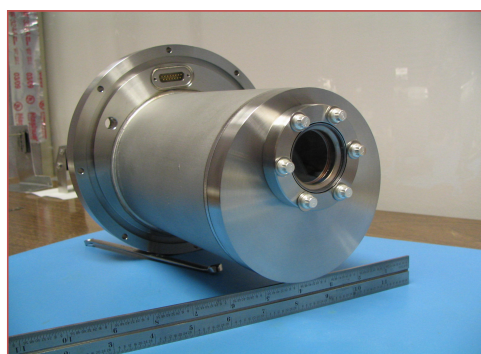
475 Figure 1: Top left is the cold finger that is held at 20° C. Top right is the CCD detector that mounts on the copper cold finger. Bottom left and right are the back and front of the assembled housing. The CCD detector is behind the window.
