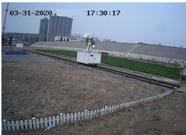
149 Fig 1 On-site photo of the surface microwave emissivity observation system 150 operating over various surfaces at the Xianghe site, China 151
