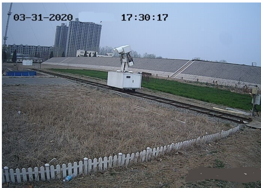
149 150 Fig 1 On-site photo of the surface microwave emissivity observation system 151 operating over various surfaces at the Xianghe site, China 152
