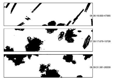
Figure 1. Examples of particle images from the Stratton Park Engineering Company Two-Dimension Stereo (2DS) probe, showing the presence of (a) column, (b) plate and (c) dendrite on 13 February 2018. Each image frame is 1.28 mm high, taken from one of the probe channels only since the other channel was not working properly on this day.
