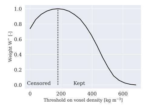
Figure A1. Example, for a reconstructed snowflake, of the distribution of the weight  $W^*$  as a function of the threshold on the voxel density content  $\rho$ . The weight is displayed here as normalized between 0 and 1. The threshold maximizing  $W^*$  is considered as optimal and it is used to censor the data to calculate geometric descriptors. A maximum could always been obtained for all the reconstructed snowflakes.
