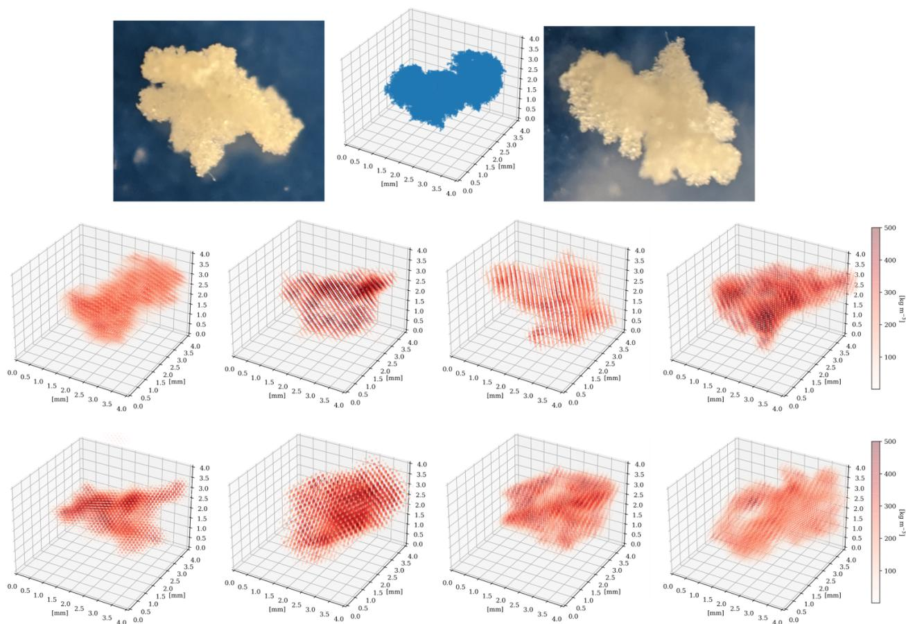
**Figure 2.** Example of the reconstruction outcome obtained while releasing eight consecutive times the same snowflake replica in the MASC measurement area. Top rows: actual photos of the replica and a pseudo-3D representation (every blue point represents a voxel filled with ice). Bottom rows: reconstructions obtained with 3D-GAN. Every point is color-coded according to the density (ice mass content) of each voxel.
