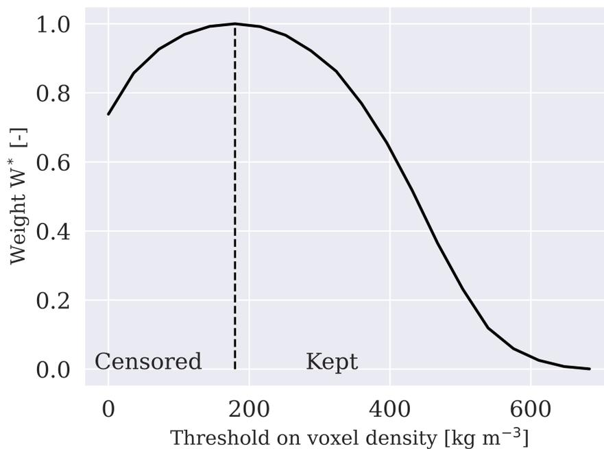
**Figure A1.** Example, for a reconstructed snowflake, of the distribution of the weight  $W^*$  as a function of the threshold on the voxel density content  $\rho$ . The weight is displayed here as normalized between 0 and 1. The threshold maximizing  $W^*$  is considered as optimal and it is used to censor the data to calculate geometric descriptors. A maximum could always be obtained for all the reconstructed snowflakes.
