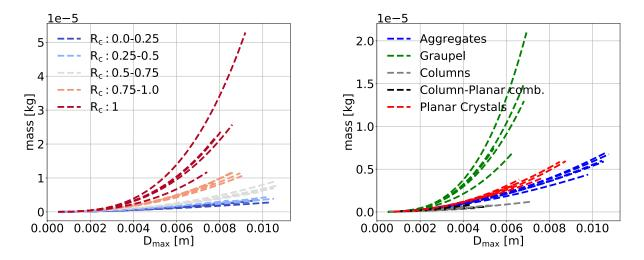
Figure 6.  $m(D_{max})$  power law relations for the data of various field campaigns, as listed in Table 5 and 4. Left: data color-coded according to riming index  $R_c$  of Praz et al. (2017). Right: data color-coded according to the hydrometeor classes, also of Praz et al. (2017). Different curves of the same color correspond to different field campaigns.
