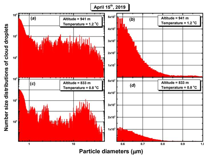
Figure 12: Detailed size distributions obtained with the standard pure water FWSCS from two PbP files of different flight lines performed on April 15<sup>th</sup>, 2109, through the same liquid cloud over southern Romania. Panels (a) and (b) correspond to the higher altitude, while panels (c), (d), show results for the lower altitude. Panels (b) and (d) focus on the sub-micrometer details of the full size distributions plotted in panels (a) and (c).
