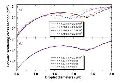
Figure 9: Enlarged view of the small-diameter range of the diagrams of Figure 8, with focus on the sub-3 µm region. (a) Horizontal shifts no larger than 100 nm may occur when the real part of the refractive index varies. (b) Wide variations in absorption (imaginary part of the refractive index) make almost no changes in the zoomed region of the FWSCS diagrams.
