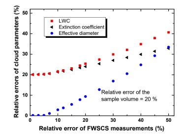
Figure 7: Relative errors of the LWC, the extinction coefficient and the effective diameter as functions of the relative error in measuring the FWSCS. Different scales have been used on the axes in order to reach a convenient aspect ratio of the figure.
