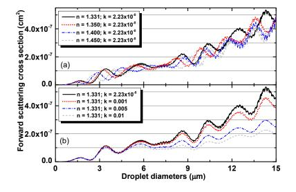
Figure 8: Computed FWSCS-diameter diagrams for the same size range, laser wavelength and angular interval of collecting scattered light, but for (a) different values of the real refractive index and (b) various degrees of absorption (as indicated by the imaginary part of the refractive index)
