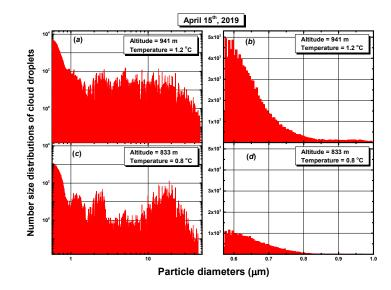
Figure 12: Detailed size distributions obtained with the standard pure water FWSCS from two PbP files of different flight lines performed on April 15<sup>th</sup>, 2109, through the same liquid cloud over southern Romania. Panels (a) and (b) correspond to the higher altitude, while panels and (c), (d), show results for the lower altitude. Panels (b) and (d) focus on the sub-micrometer details of the full size distributions plotted in panels (a) and (c).
