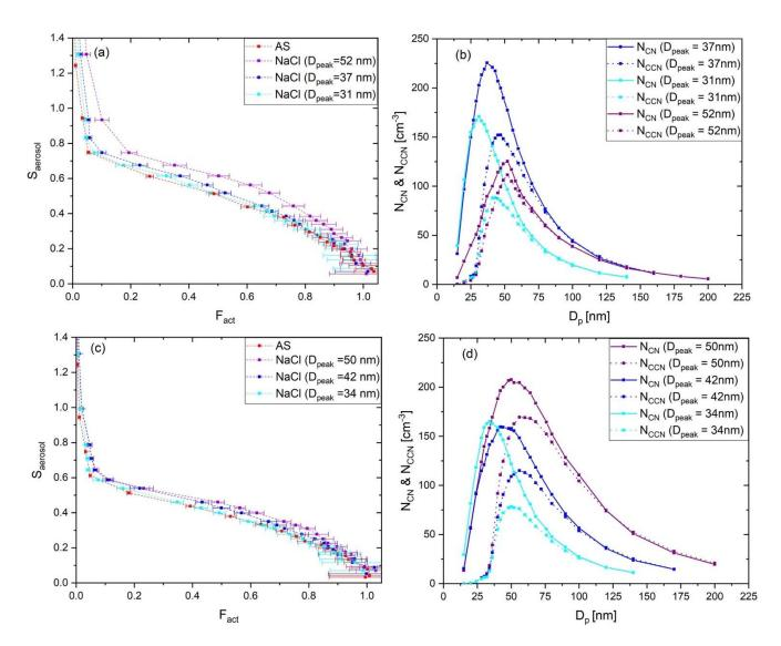
Figure 5: Calibration curves of ammonium sulfate and sodium chloride for (a) dT=10 K and (c) dT=8 K and number size distribution 525 of  $N_{CN}$  and  $N_{CCN}$  for sodium chloride particle for (b) dT=10 K and (d) dT=8 K.
