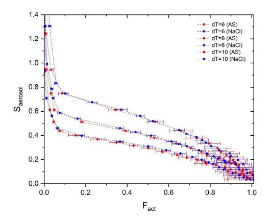
Figure 2: Calibration curves ( $F_{act} - S_{aerosol}$ ) for three different T gradients (dT = 6, 8, and 10 K) with ammonium sulfate (red) and 510 sodium chloride (blue) particles.
