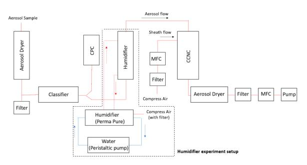
505 Figure 1: Schematic plot of a broad scanning supersaturation cloud condensation nuclei counter (BS2-CCN) system. An additional setup marked with dashed line is for a humidifier experiment.
