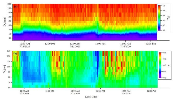
Figure 10: Time series of (a)  $F_{act}$  and (b)  $\kappa$  distribution of BS2-CCN measurement for 0.63% S (dT=8 K) condition. Measurement period was 13 July – 16 July 2020.
