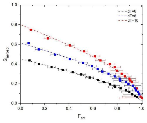
Figure 8: Experimental data (square dot with error bar) and fitting curves (dashed lines) for three different dT conditions (dT = 6 (black), 8 (blue), and 10 K (red)). Ammonium sulfate particles are used for calibration.
