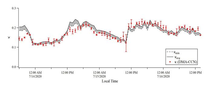
550 Figure 11: Time series of hourly averaged  $\kappa$  values for DMA-CCN (red dots, bar indicates the standard deviation of  $\kappa$ ) and BS2-CCN (grey shaded area for the range between  $\kappa_{avg}$  (black solid line) and  $\kappa_{low}$  (black dashed line)) measurements. The  $\kappa_{high}$  is excluded in this figure.
