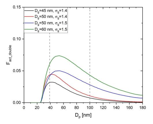
520 Figure 4: Activation fractions by doubly charged particles ( $F_{act\_double}$ ) for variant particle size distributions. Information of each particle size distribution is presented in the legend of the figure.
