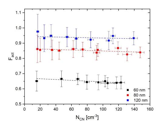
Figure 6: Average and standard deviation (error bar) of F<sub>act</sub> depending on the number concentration N<sub>CN</sub> for 60 nm (black), 80 nm (red) and 120 nm (blue) of ammonium sulfate particle under the dT=7.7 K (0.6% S) condition. Dashed lines indicate linear regression
