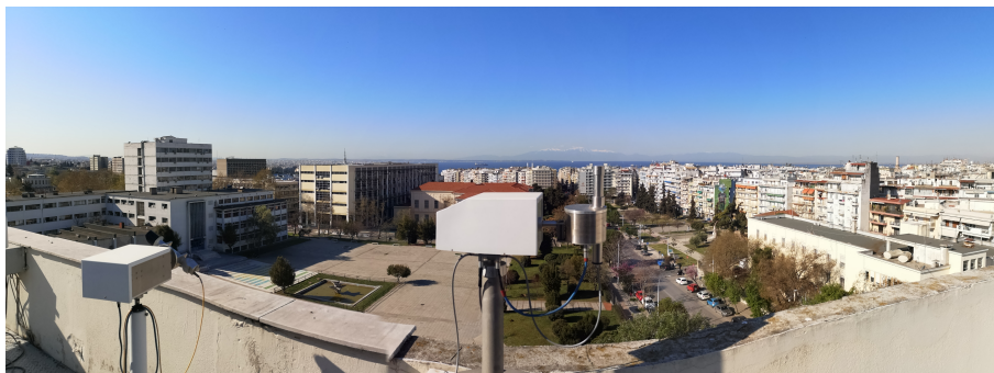
Figure 1. The Phaethon MAX-DOAS system in the middle and a panoramic view (East - South - West) of the measurement site.
