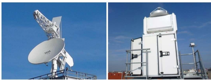
Figure 1: C-band POLDIRAD weather radar (left, photo: Martin Hagen) and Ka-band MIRA-35 cloud radar (right, photo: Bernhard Mayer).
