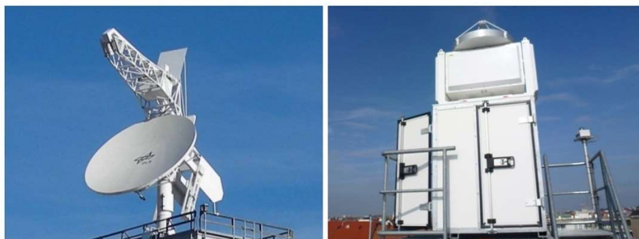
Figure 1: C-band POLDIRAD weather radar (left, photo: Martin Hagen) and Ka-band MIRA-35 cloud radar (right, photo: Bernhard Mayer).
