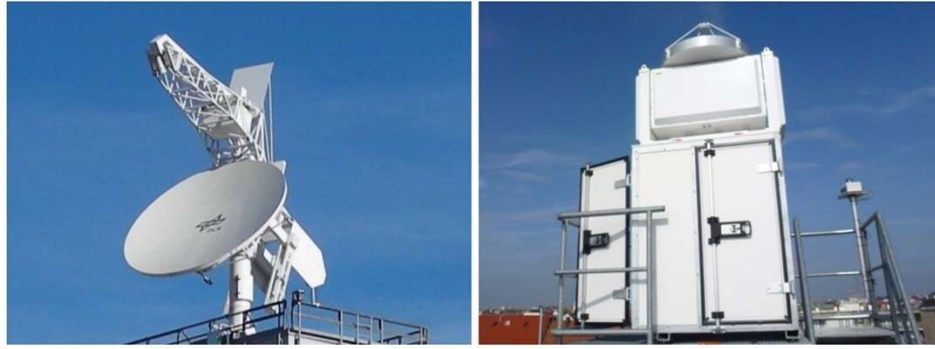
Figure 1: C-band POLDIRAD weather radar (left, photo: Dr.rer.nat. Martin Hagen) and Ka-band MIRA-35 cloud radar (right, photo: Prof. Dr. Bernhard Mayer).
