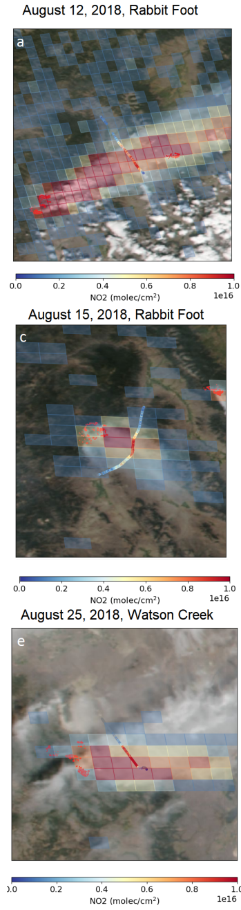
Figure 10. Comparison between the BB-FLUX aircraft measurements (CU-DOAS, 10 s averages are shown together with the corresponding standard deviation) and TROPOMI NO 2 VCDs (VCD EC ). The maps with the satellite pixels and aircraft transects are shown in the panels on the left (a, c, e). The overlay is a VIIRS true colour image with the MODIS fire hotspots, shown as red dots (obtained from NASA Worldview; https://worldview.earthdata.nasa.gov/ ). The plume age for pixels with VCD > 1 \times 10^{15} molec/cm 2 is shown in the panels on the right (b, d, f) for the TROPOMI VCD EC (grey) and the CU-DOAS VCDs (yellow, orange and red). The time of the observations is displayed in the legend.
