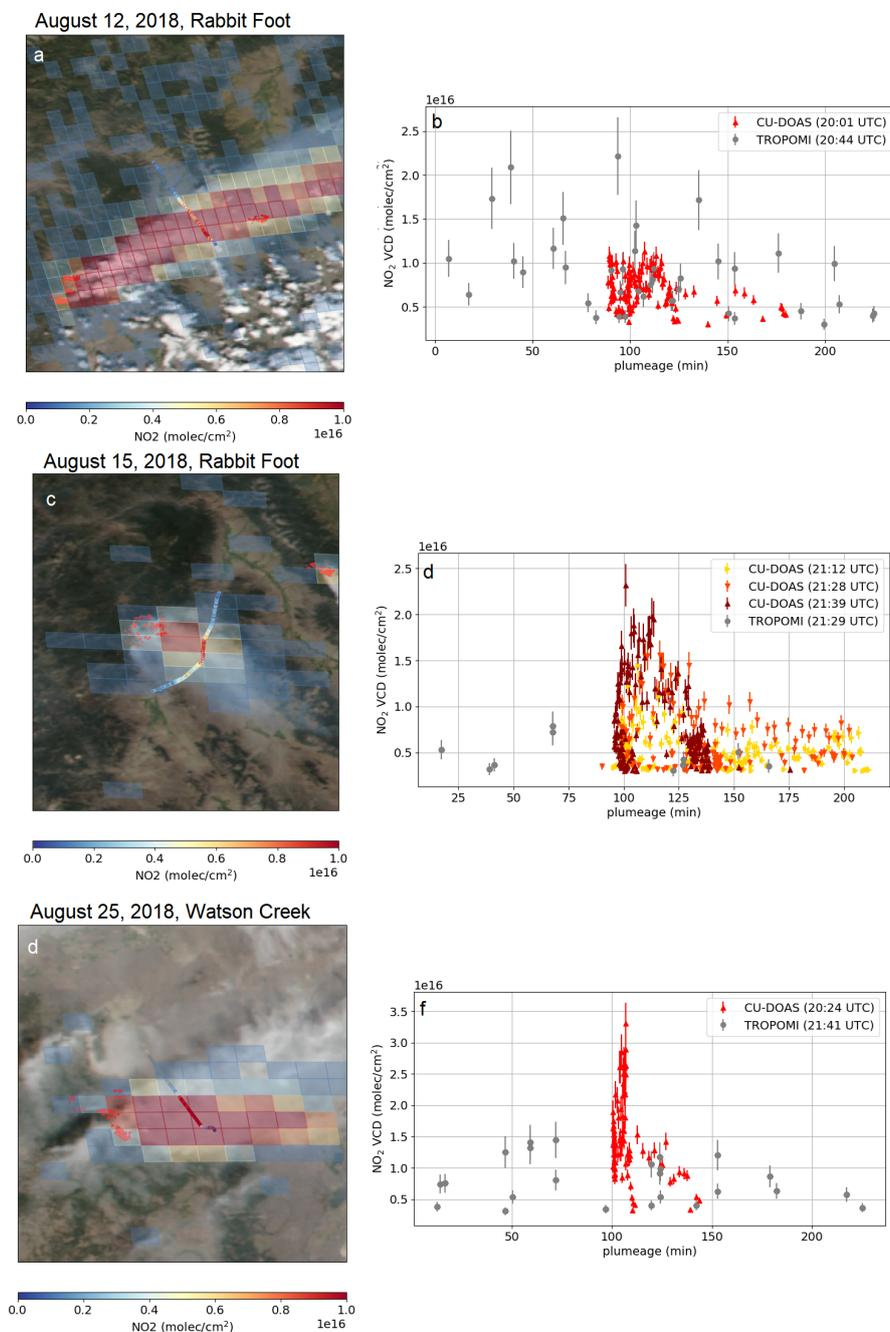
**Figure B2.** Same as Fig.10, but for the TROPOMI  $VCD_{KNMI}$  instead. The mean difference is  $-1.75 \pm 4.51 \times 10^{15}$  molec/cm<sup>2</sup> (-26 %) and  $2.21 \pm 1.56 \times 10^{15}$  molec/cm<sup>2</sup> (32 %) for the Rabbit Foot fire on August 12 and 15, respectively.
