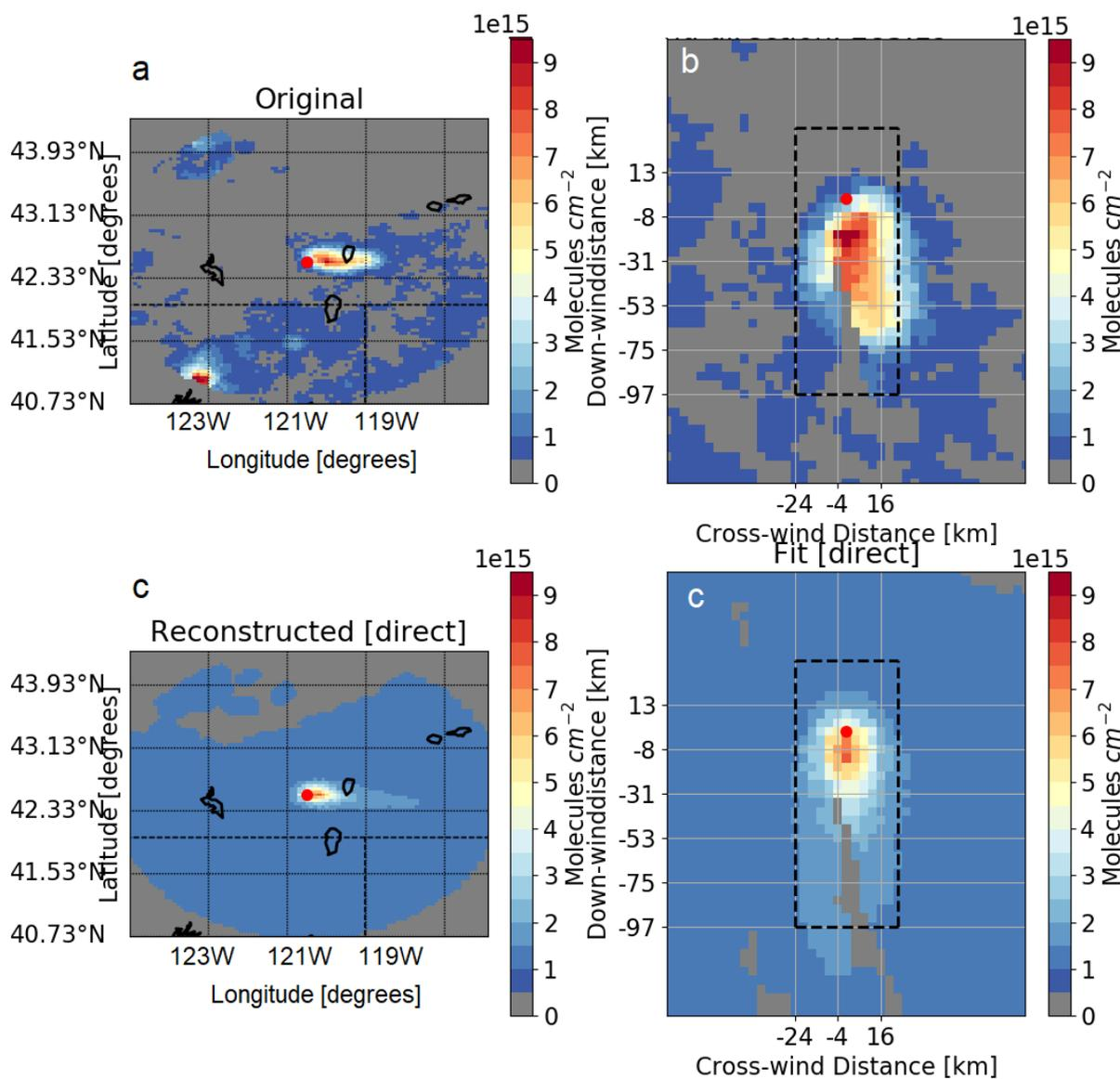
**Figure 4.** Example of the EMG method for the Watson Creek fire on August 25, 2018 at approximately 43.5°N, 120.7°W in Oregon, US (same as in Fig. 3). The TROPOMI NO<sub>2</sub> observations ( $VCD_{EC}$ ) are shown in a latitude/longitude and upwind/downwind domain in panels (a) and (b), respectively. The fitted VCDs using the EMG are shown in panels (c) and (d) in the longitude/latitude and upwind/downwind domain, respectively.
