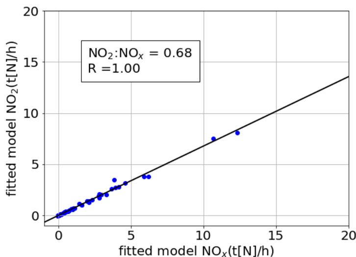
**Figure 6.** Fitted emissions derived using the EMG method for the synthetic  $\text{NO}_2$  and  $\text{NO}_x$  ( $\text{NO}_2+\text{NO}$ ) VCDs, suggesting a  $\text{NO}_2:\text{NO}_x$  ratio of 0.68 should be used for the conversion, the fitted  $\text{NO}_2$  and  $\text{NO}_x$  emissions are perfectly correlated ( $R = 1$ ).
