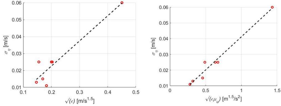
**Figure 4:** Plots of the relationship of the lidar spectral noise standard deviation  $\sigma_\eta$  with the square root of the energy dissipation rate and the product of it with the mean wind speed, respectively.
