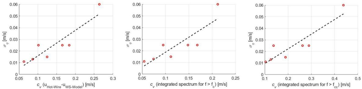
**Figure 3:** Plots of the relationship of the lidar spectral noise standard deviation  $\sigma_\eta$  with the coefficient of variation  $c_v$  calculated in different ways; Left: Difference between the modelled lidar time series (only Lorentzian filter without added noise) and the hot-wire time series. Middle: Integrated coefficient of variance of the hot-wire spectrum from  $f_c$  to infinity. Right: Integrated coefficient of variance of the hot-wire spectrum from  $f_{cc}$  to infinity.
