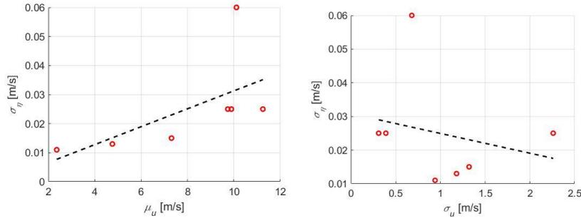
**Figure 2:** Plots of the relationship of the lidar spectral noise standard deviation  $\sigma_\eta$  with the mean wind speed  $\mu_u$  and the standard deviation  $\sigma_u$ , respectively.
