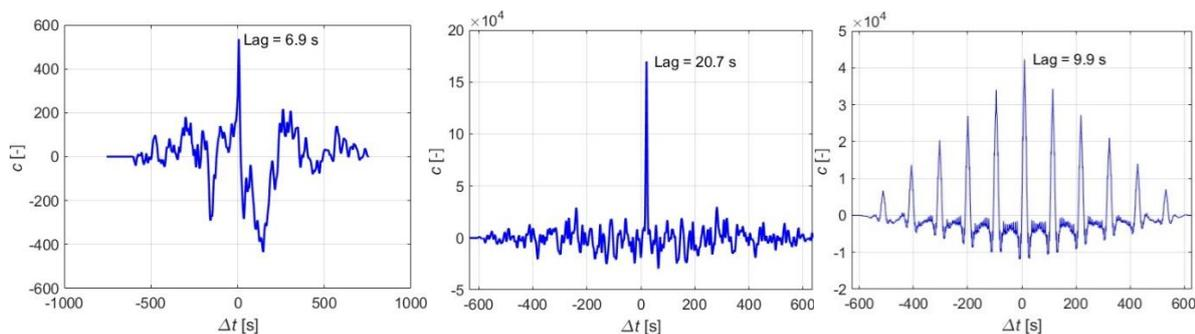
**Figure 1:** Plots of the cross-correlation function between lidar and hot wire time series for three cases (1a, 1b and 2c), used for the temporal synchronisation.
