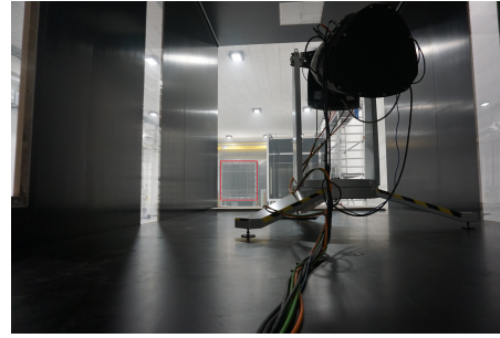
Figure 1. The open jet wind tunnel including the active grid at the nozzle. Figure 2. View into the wind tunnel from the perspective of WindScanner 1.
