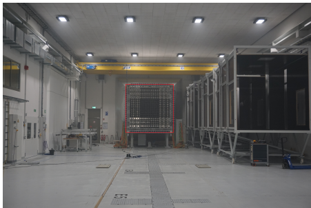
Figure 1. The open jet wind tunnel including the active grid at the nozzle.
