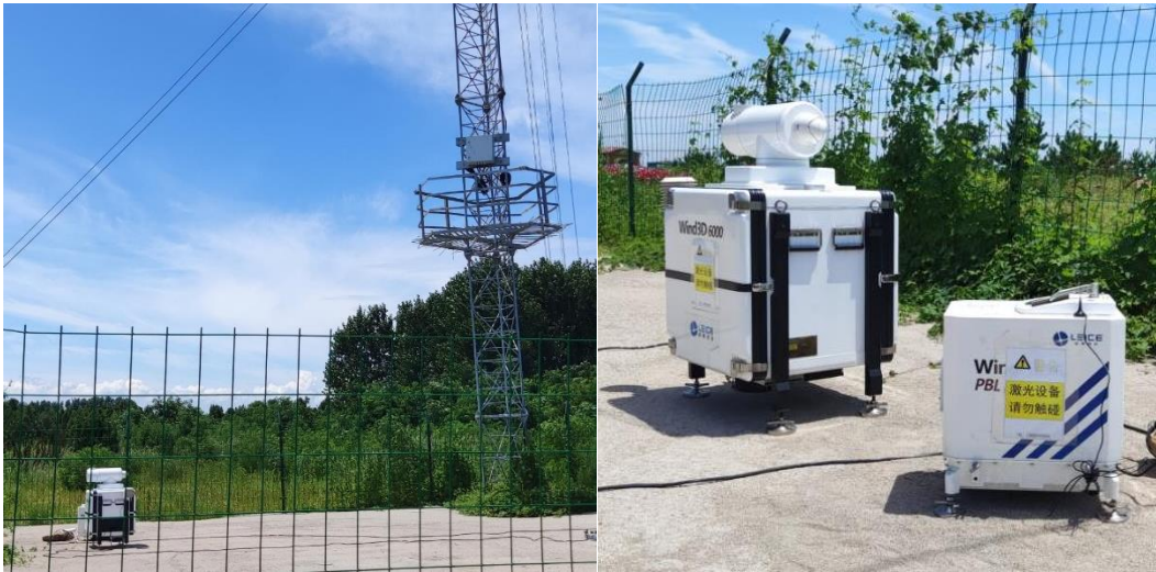
Figure 2. Photos of the CDLs and the mast that mounted cup anemometers and wind vanes at site Haiyang.
