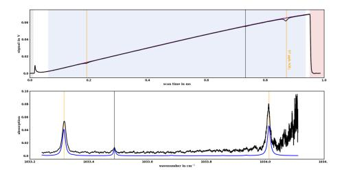
As in Figure 10 in the paper, the upper panel shows the detector signal for one laser ramp, and the lower panel shows the spectrum in absorption space. The blue line does not show a fit but rather a HITRAN based spectrum for the 57 ppb NH<sub>3</sub> mixing ratio in the standard that was used.
