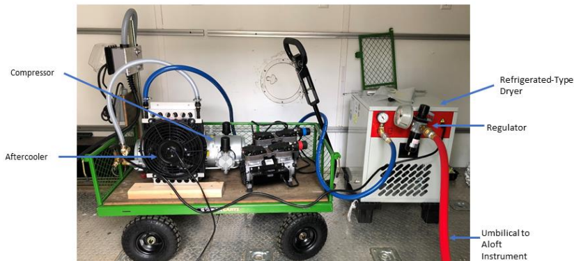
Figure 5. Dry air generation equipment including compressor, aftercooler, dryer, regulator, and umbilical hose.
