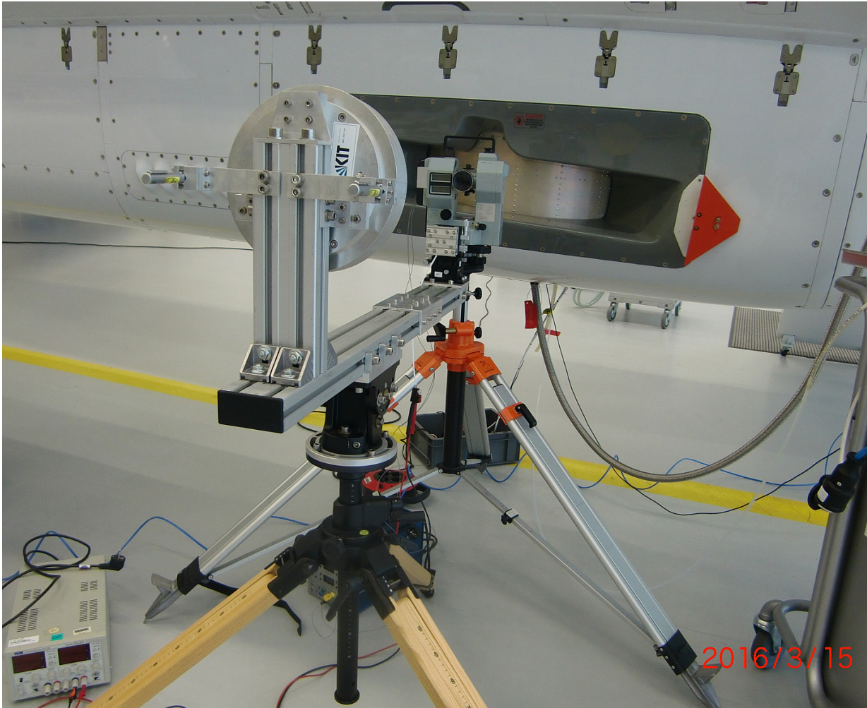
Figure 12. Pointing calibration optics with an off-axis paraboloid mirror which is delivering parallel beams with a broadband infrared light source in front of the GLORIA instrument (golden) integrated in the belly pod of HALO in Oberpfaffenhofen. In between the theodolite during the adjusting phase of the beams.
