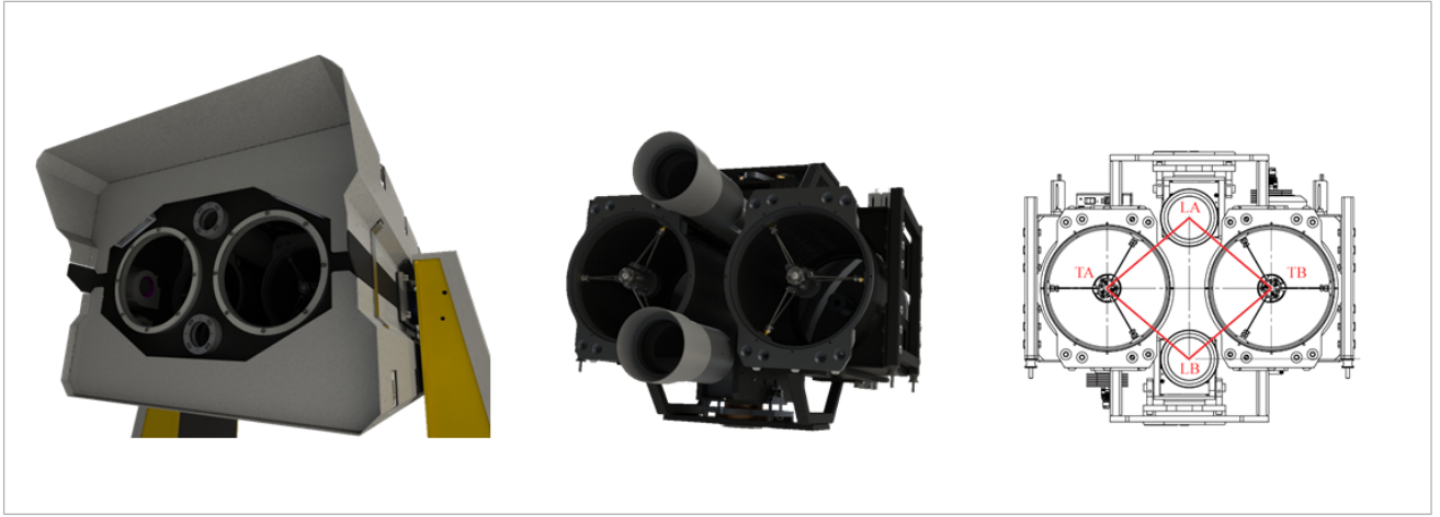
Figure 3. The lidar head. Left: Cover of the lidar head, showing the windows in front of the two lasers and the two telescopes. Middle: Photorealistic image of the internal parts of the head, showing the lasers and their beam expanders, the telescopes and the rest of the detection units. Right: Front view of the head, showing the diamond-shaped layout of the lasers (LA and LB) and telescopes (TA and TB).
