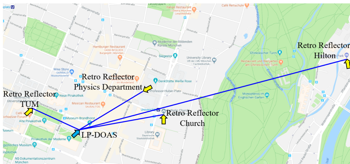
Figure S1. The setup of the LP-DOAS system on the MIM's rooftop with its four optical paths towards TUM N5 building, LMU physics building and Hilton hotel (Figure from Zhu et al., 2020). The retro reflector at the Church was only installed in January 2017 and was not available in 2016 during the MuNIC campaign. Map data (c)Google maps.
