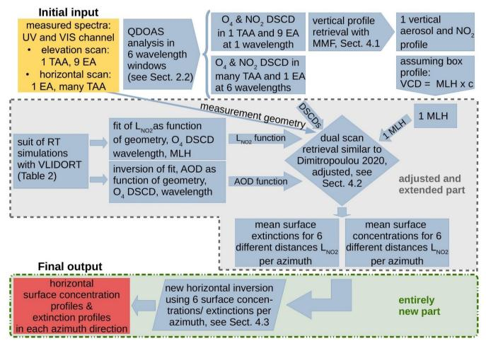
Figure 3. Mapping MAX-DOAS technique flow chart.
