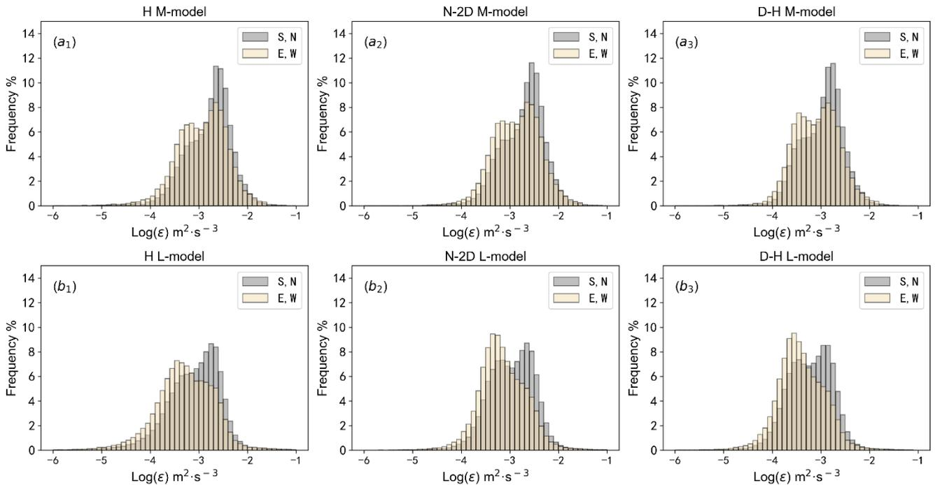
235 Figure 8. Distribution of  $\epsilon$  in the middle and low mode of the Beijing MST radar in the range of 3–7.8 km from 2012–2014: ( $a_1$ – $a_3$ ) distributional characteristics of  $\epsilon$  in the H model, N-2D model and D-H model (mid mode); ( $b_1$ – $b_3$ ) as in ( $a_1$ – $a_3$ ) but for low-mode data. The gray bars are the result of a north and south beams, the yellow bar are based on the east and west beams.
