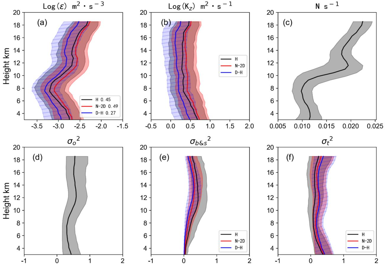
Figure 7. Profiles of (a)  $\epsilon$ , (b)  $K_z$ , (c) B-V frequency, (d) observation spectrum width, (e) beam and shear broadening, and (f) spectrum width caused by turbulence. The solid line is the median and the shaded area is the upper and lower quartiles. In panels (a, b, e, f), the black/red/blue solid lines and shaded areas represent the median and upper and lower quartiles of the H model/N-2D model/D-H model, respectively.
