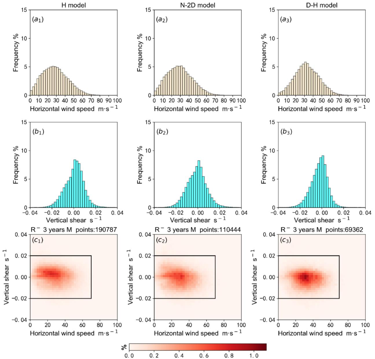
Figure 4. Frequency distribution of (a<sub>1</sub>–a<sub>3</sub>) horizontal wind speed and (b<sub>1</sub>–b<sub>3</sub>) the vertical shear of horizontal wind speed, along with (c<sub>1</sub>–c<sub>3</sub>) the two-dimensional frequency distribution characteristics
