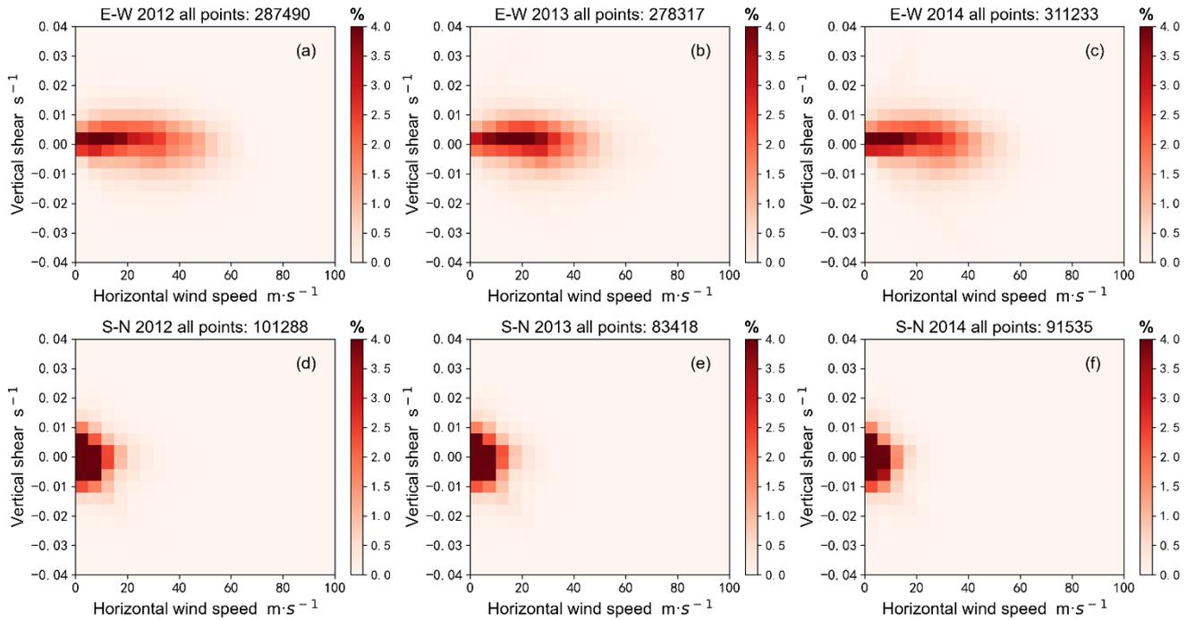
Figure R-10. Two-dimensional frequency distribution characteristics of horizontal wind speed and vertical shear of horizontal wind speed within the height range of 3–19.8km above the Beijing MST radar station from 2012 to 2014. (a)(b)(c) The east-west component of horizontal wind, (d)(e)(f) The north-south component of horizontal wind.
