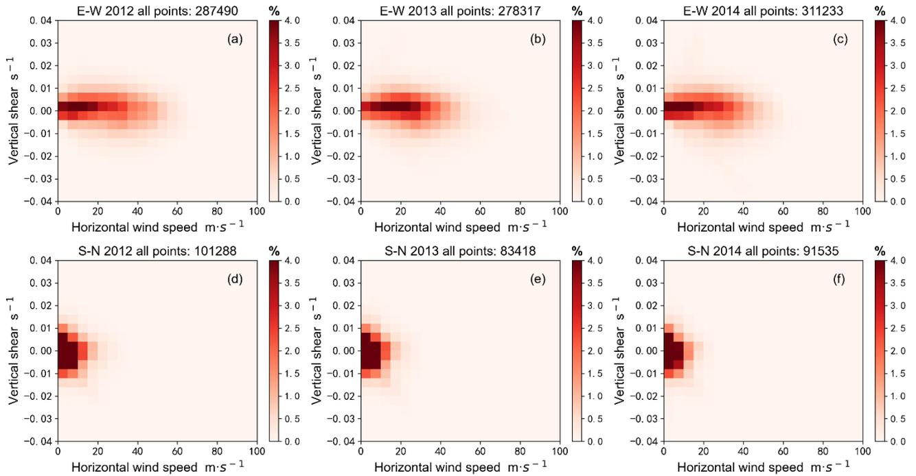
125 Figure R-2. Two-dimensional frequency distribution characteristics of horizontal wind speed and vertical shear of horizontal wind speed within the height range of 3–19.8km above the Beijing MST radar station from 2012 to 2014. (a)(b)(c) The east-west component of horizontal wind, (d)(e)(f) The north-south component of horizontal wind.
