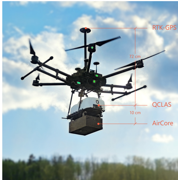
Figure 1. The embedded UAV system used for CH 4 detection: the QCLAS analyzer and the active AirCore sampling system are mounted below a Matrice 600 DJI hexacopter equipped with a RTK-GPS system.
