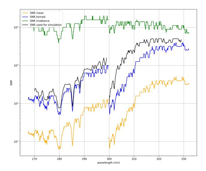
Figure 1: SNRs for a single (binned) TROPOMI pixel (orbit 5005) at 51° latitude, 154° longitude, 56° SZA, 9° VA and 70° AA with an albedo of 0.1. In green the irradiance SNR is given, which is binned for 8 pixels in UV2. The binned (1x8 UV1, 8x8 UV2) radiance SNR is shown in blue and the mean radiance SNR is given in yellow. The (binned) SNR, which was used for the sensitivity study with simulated spectra shown in Fig. 2 in the paper, is shown in black.
