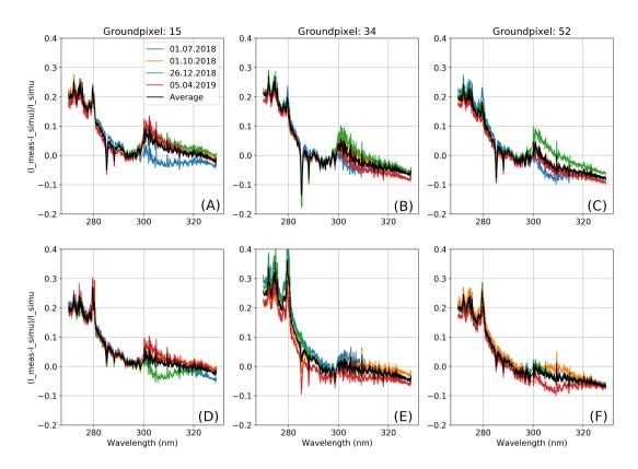
Figure 5. Relative differences between the measured and simulated radiances for three detector pixels (viewing angles). Upper panels: cloud-free tropical pixels ( $-50^{\circ}$  to  $20^{\circ}$  latitude). Lower panels: cloud-free extratropical pixels ( $-50^{\circ}$  to  $-30^{\circ}$  and  $30^{\circ}$  to  $50^{\circ}$  latitude). Black curves represent mean values of four orbits.
