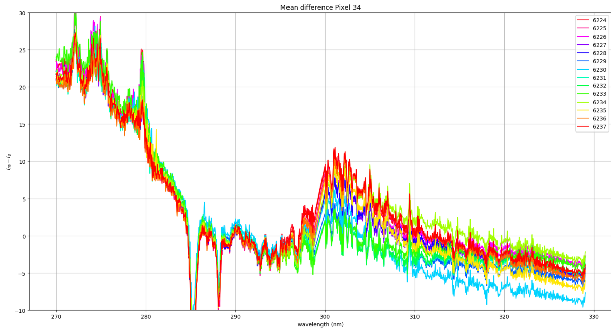
Figure 2: Re-calibration spectra (relative mean difference between measured and simulated spectra) for a full day 26.12.2018 of TROPOMI for pixel nr 34.
