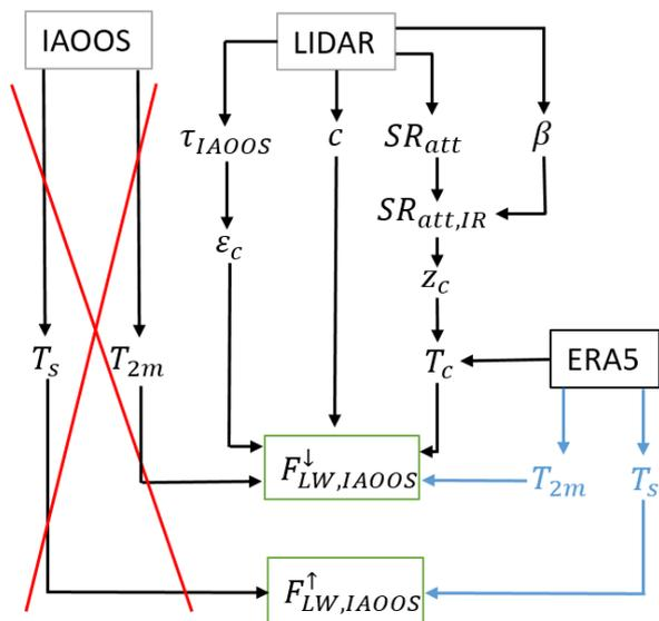
Flowchart describing the method to get the downward LW flux  $F_{\downarrow LW}$  from the observations onboard the IAOOS buoy (temperature and lidar measurements).  $T_s$  and  $T_{2m}$  are over this period (April-June 2015) are instead taken from ERA5 (blue) because there are not available from the IAOOS buoy due to instrumental issues (red cross).  $\tau_{IAOOS}$  is obtained from the flowchart describing the retrieval of SW fluxes.
