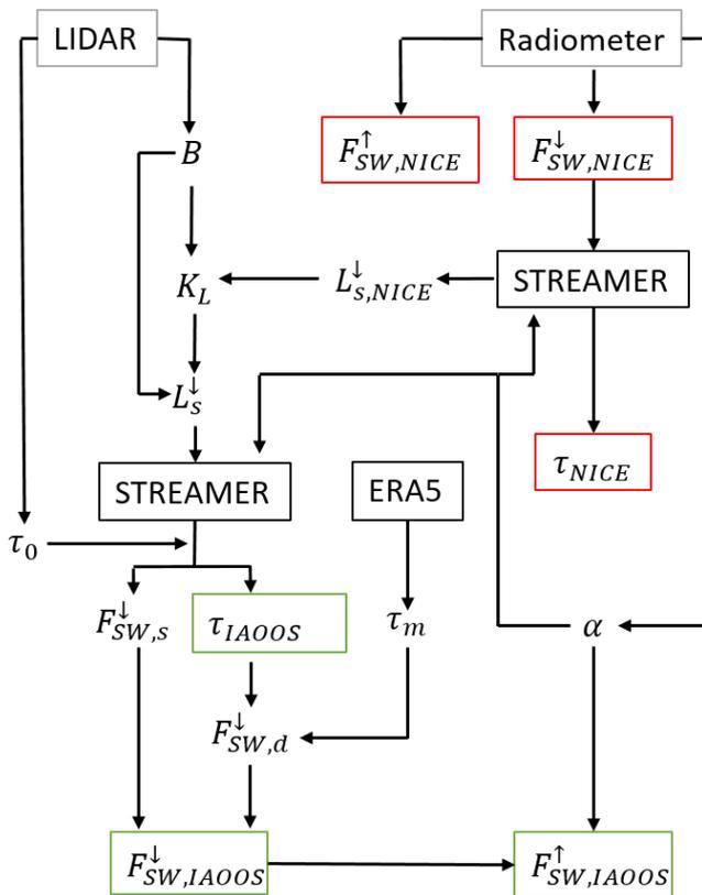
Flowchart describing the method to get the downward SW flux  $F_{\downarrow SW}$  from the solar background  $B$  measured by the lidar. The estimated optical depth  $\tau_{IAOOS}$ ,  $F_{\downarrow SW}$  and  $F_{\uparrow SW}$  in green are compared to their observed counterparts from N-ICE measurements in red.  $\tau_{IAOOS}$  is then used to estimate the downward LW flux.
